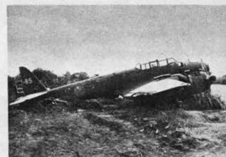
Captured Irving has new short cockpit, smooth dorsal line from cockpit to tail.
